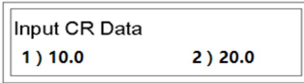
Initially in this Mode, cursor flashes in Line **1)**, (which means data can be input), input the data, from 0-650.0, accurate to one decimal place.
