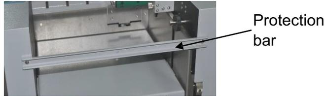
The first thing after unpacking and putting machine on table is to uninstall the protection bar.
