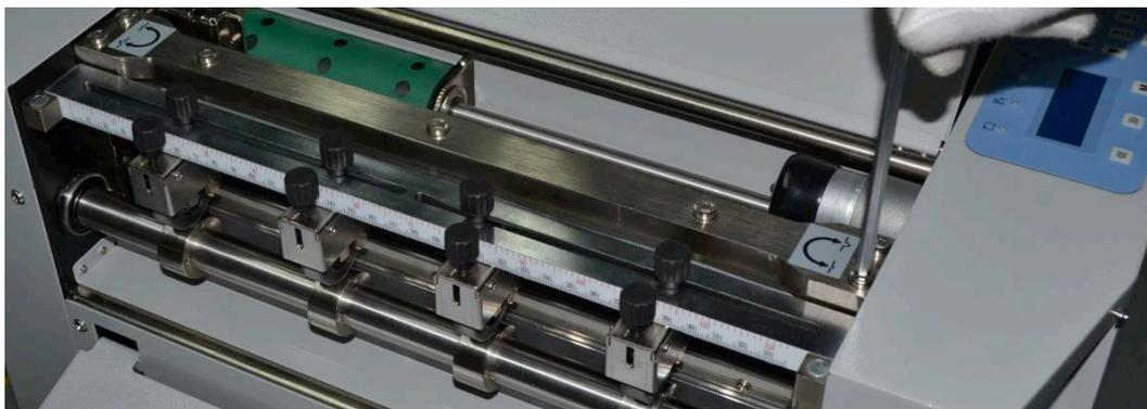
Find 4 screws on both side, turn the Allen screw according to the label
