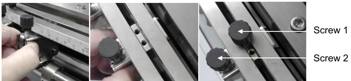
Screw 1 to fix the blade with the machine.
