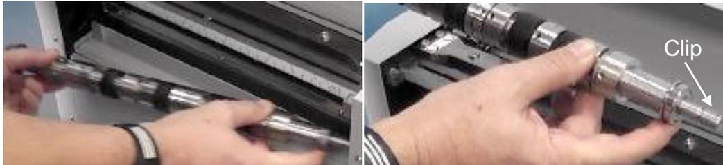
4. After anvil is mounted again, reinstall the shaft, so to the clip.
