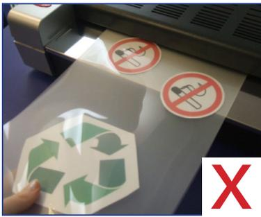
Never laminate small, cut-up pieces without using a Lifejacket® or you risk jamming and damaging your laminator (this will not be covered under warranty)
