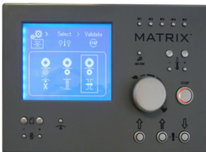
Ensure for foiling the bottom temperature is set to zero (off).
