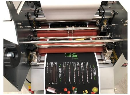
Enter the display encapsulating/foiling mode (page 7-8 for display navigation) and turn on the bottom roller temperature (set at minimum of 10 degrees higher than the top roller). Load the films as normal. You do not need the perforator or angle wheels. Increase the pull roller pressure to between 0.4-0.6psi. Ensure the top and bottom films are correctly aligned.
