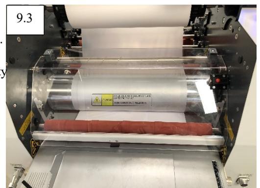
9. Manually push the feed roller down and insert another card (9.1). While pushing the card press the foot pedal, moving the sheet into the rollers until it reaches the feed gate (9.2). Put on the safety guard and push in the latch (9.3).
