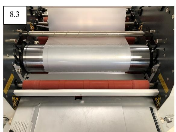
8. While pushing the card press the foot pedal (8.1), moving the sheet into the rollers until it reaches the nip (8.2) and put the feed gate plate and thumb screws back into position (8.3).
