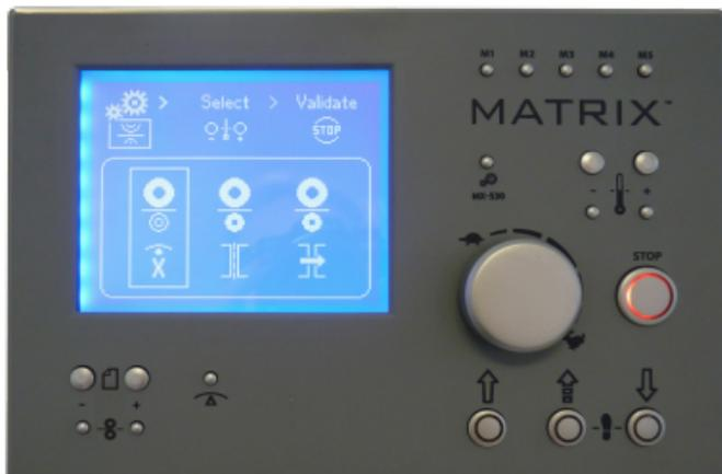
As explained on previous page press the function/settings key to enter screen, use the temperature buttons to select mode and press stop to enter.
