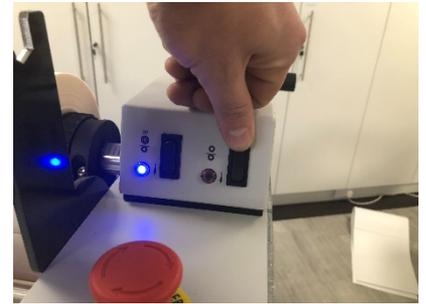
If your sheet is curling upwards you need to increase the anti-curl and decrease if curling down. To change the anti-curl setting release the pressure on the pull roller, change setting and put the roller back down. Ensure the anti-curl mechanical setting matches the display setting.
