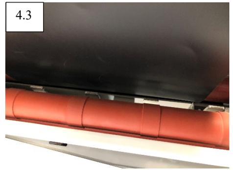
4. Push the feed card down in between the bottom laminating roller and grey support plate (4.2 & 4.3). Ensure the Matrix Duplex writing is facing the feed table (see below 5.1 & 5.2).
