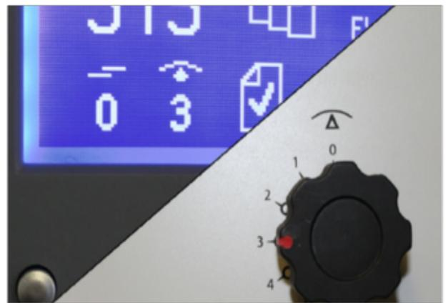
Ensure the perforator wheel is set over the laminating film within 5mm from the edge and anti-curl mechanical setting matches the display setting. Depending on the media and material being used you might require both angle wheels, ensure the angle wheel on the left is angled more than the one directly next to the perforator. If you have Pneumatic splitting pressure this might need to be increased, for single sided is usually between 0.2-0.4psi and double sided between 0.4-0.6psi.
