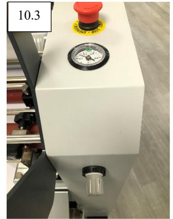
10. Turn the bottom perforator anti-clockwise until loose (10.1). Depending on the media and material being used you might require both angle wheels (10.2) and more pressure on the pneumatic splitting (10.3). If the second angle wheel is needed ensure the angle wheel on the left is angled more than the one directly next to the perforator. Pneumatic splitting pressure for single sided is usually between 0.2-0.4psi and double sided between 0.4-0.6psi.
