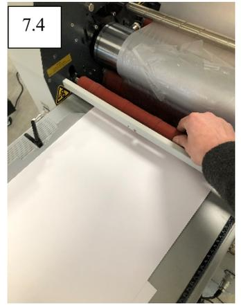
7. Pull the feed sheet up onto the feed table (7.1) and remove. Cut the film to leave a clean edge (7.2) and stick it to the top laminating film (7.3). Manually push the feed roller down and insert a thick 300gsm plain card (7.4).
