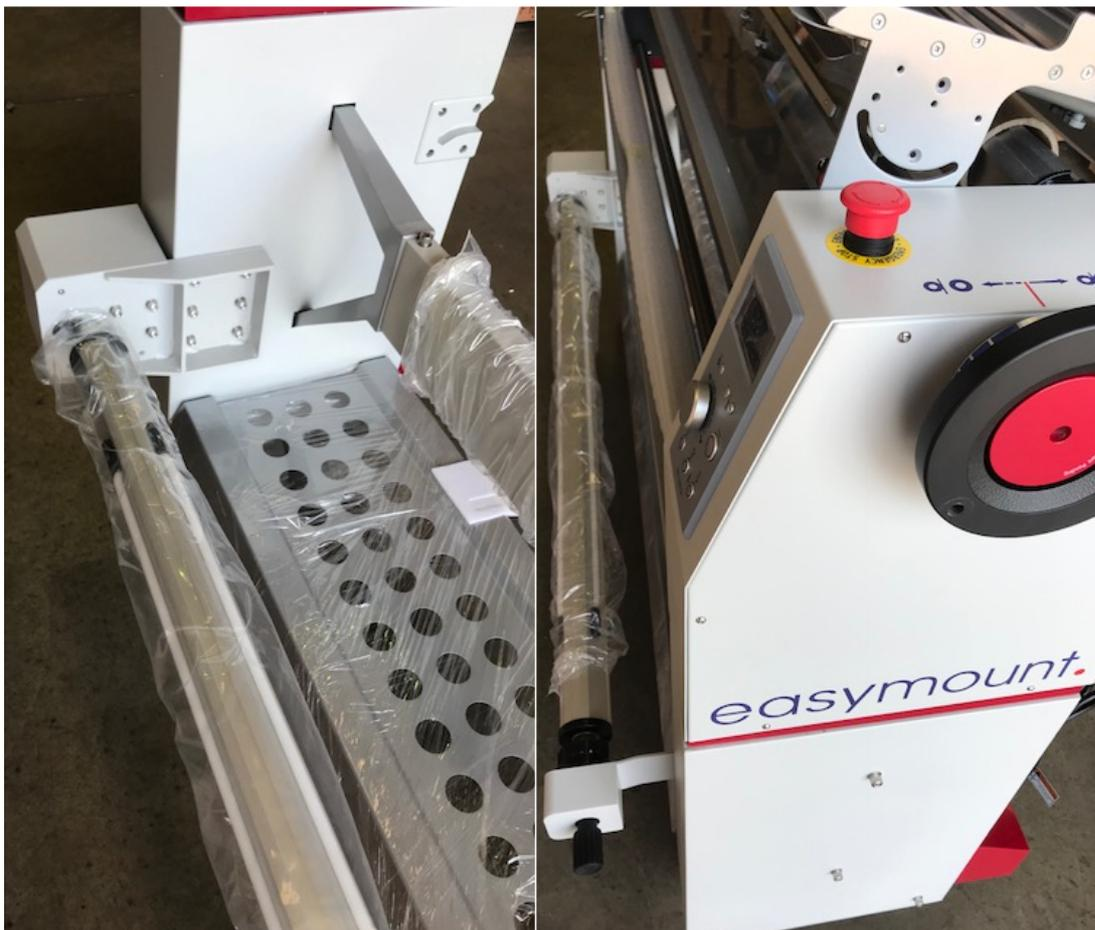
Remove Both Side Covers, Handle and Rubber Support for the Quartz Heating Element. Insert Quartz Heating Element and Re-attach the Blue Rubber Support
