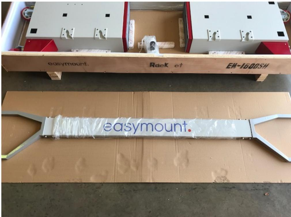
Using 2 x Stand Bolts secure the 2 x Bottom Support Beams to the Left Stand Frame and place the Centre Support beam in the Centre Slots.
