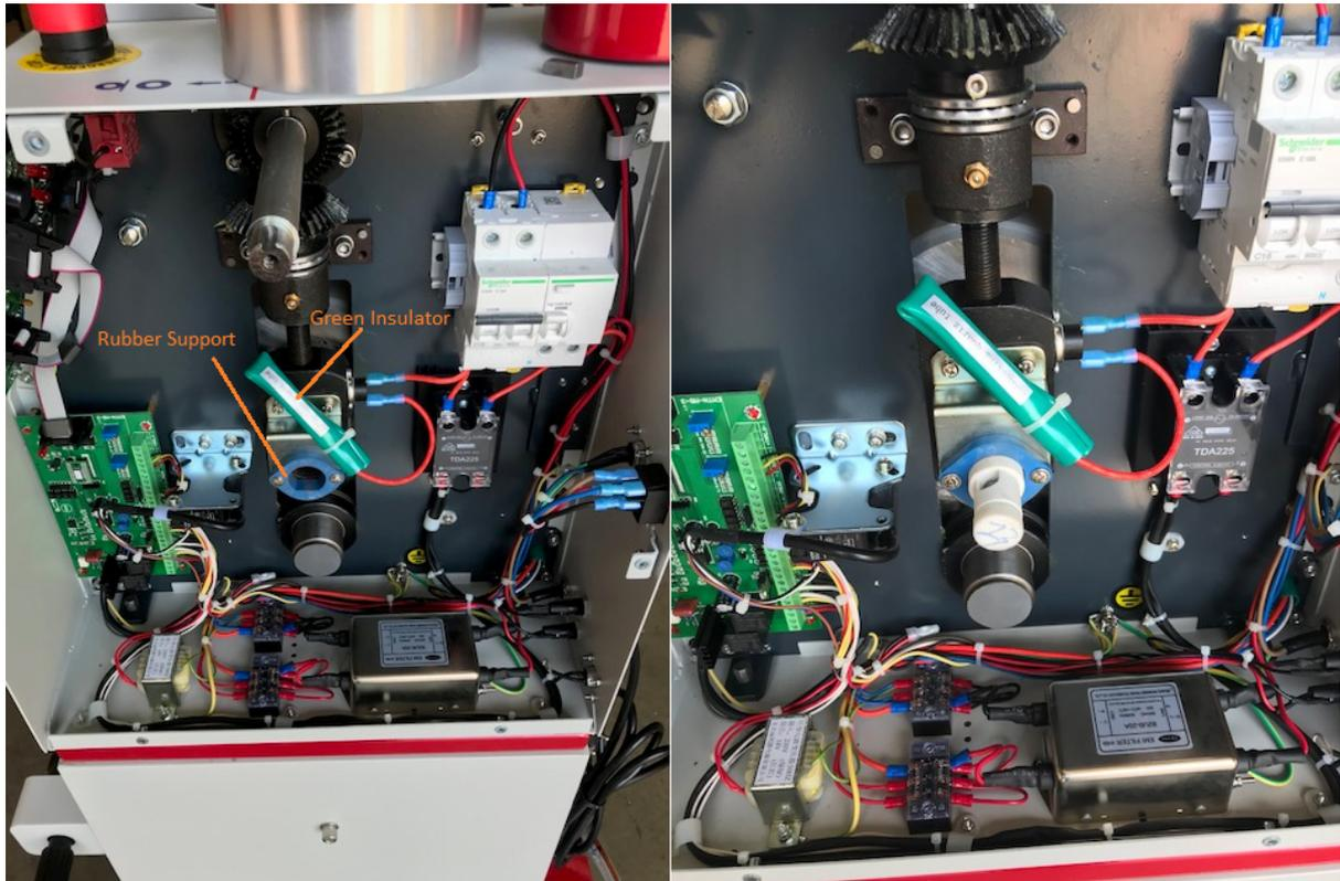
Remove the Green Insulator and attach the terminal to the element and both sides.
