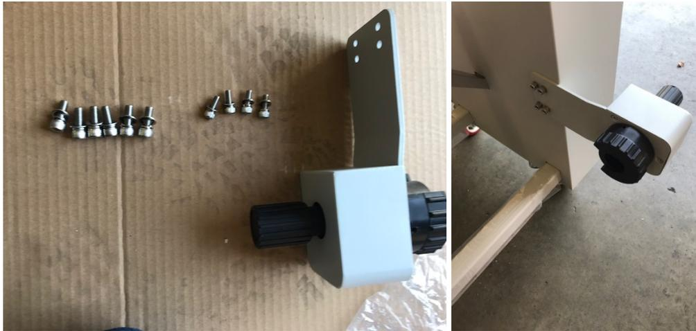
Keep the 6 x bolts safe in the photo safe until you have un-crated the Laminator.
