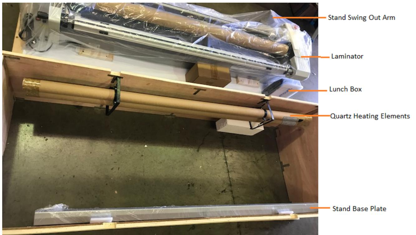
Put the Stand Base Plate on the base of the stand.
