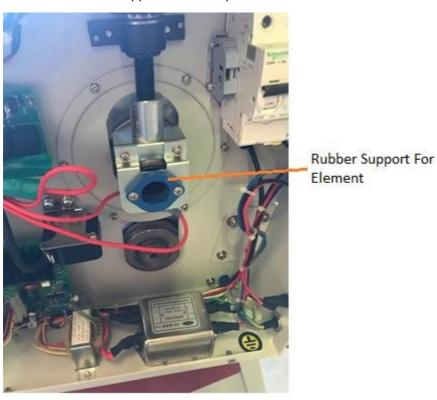
Remove the Green Rubber sleeve on the left and right sides and attach the wire to each end of the element, ensuring there is a washer on either side of the terminal as shown in the pictures below.
