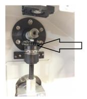
Once the rollers are set, follow the instructions in reverse to put the machine back together.
