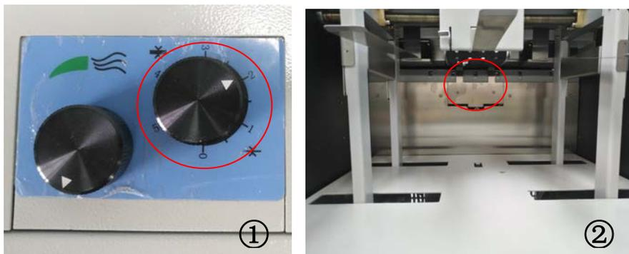
As shown in the following figures. Turn the knob anticlockwise can increase the gap while clockwise decrease the gap. When the sheets double fed, we need to decrease the gap. When the sheets get stuck at the entrance, we should increase the gap.
