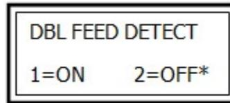
**Notes:** The double feed detecting sensors are optional. If there are no double feed detecting sensors on the machine but the double feed detect is on, it will come up the error message.
