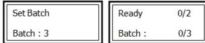
**Notes:** When the sheet quantity is less than the setting, the machine will stop. Then after we place more sheets on the table, it will continue the last job.
