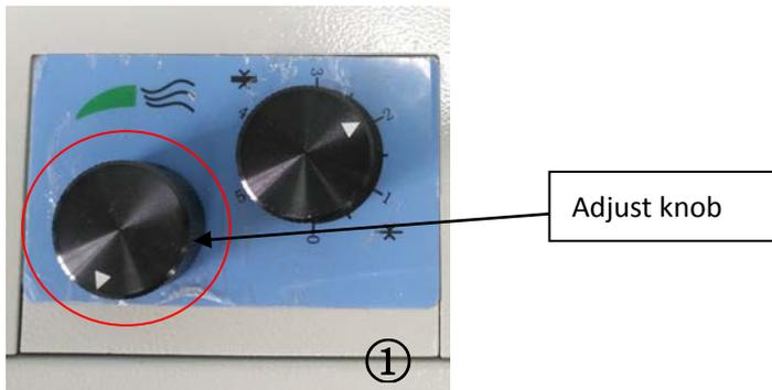
Turn the knob clockwise can weaken the blowing. When we run smaller and thinner sheets, we can try weakening the blowing to make it fed smoothly and stably.
